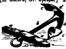
Anchor. a A Stock; b Shank; c E Flukes; d d Arms.
