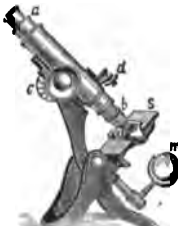
Microscope. a Eyepiece; b Objective; c Rack and Pinion for coarse adjustment of focus; d Screw for fine adjustment; m Mirror; s Stage.
