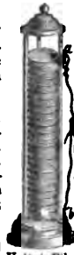
Voltaic Pile. a Upper Disk of Zinc; b Lower Disk of Copper or Silver.
