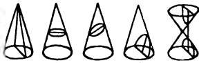
Conic Sections (the right lines and circle being sometimes included). a Right lines; b Circle; c Ellipse; d Parabola; e Hyperbola.
