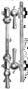
Water Gauge, a. Wall of Boiler; b. Glass Tube of Water Gauge in which the Water stands at the Level of that (c) in the Boiler; c. Cocks.
